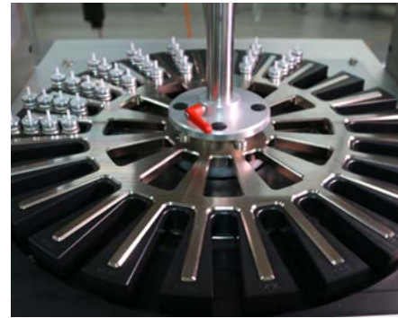
Easy assembly and disassembly of therotary star wheel
